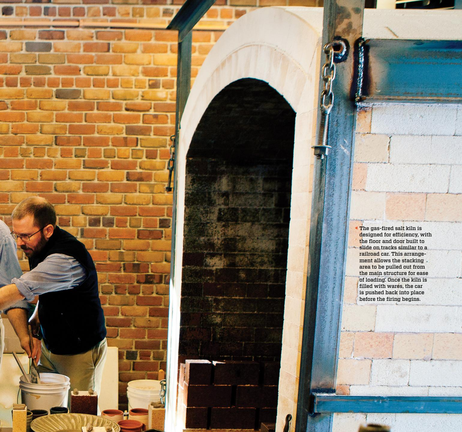
◀ The gas-fired salt kiln is designed for efficiency, with the floor and door built to slide on tracks similar to a railroad car. This arrangement allows the stacking area to be pulled out from the main structure for ease of loading. Once the kiln is filled with wares, the car is pushed back into place before the firing begins.
